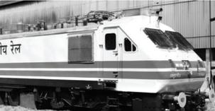
Express. This locomotive has also been provided with Crew Voice and Video Recording System (CVRS) for Onboard Driving data Recording and Analysis. Cameras with microphones are provided at the critical positions inside & outside the locomotive to record the voice and audio signals for post event analysis with storing the data into digital format. (EOIC)
