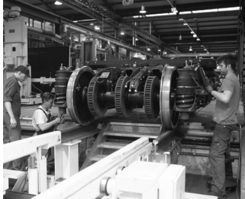
Workers perform maintenance work on a train's running gear at an Austrian railways OeBB service facility in Vienna, Austria.
