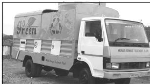
Picture shows a mobile Sewage Treatment Plant parked along the road near Dollygun. The customized mobile treatment plants are used by some top hotels and resorts in the city and tourist hotspots like Havelock and Neil Island for treatment of waste water and sewage. (EOI Pix)
